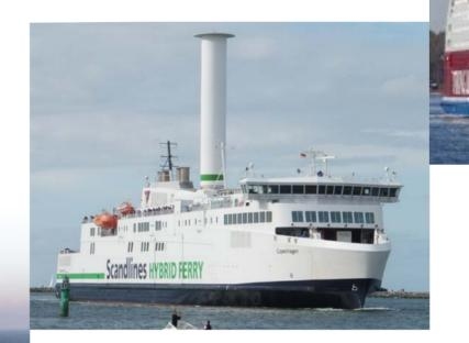
Ship name: Copenhagen Type: RoPax Ferry Vessel data: LOA 169.5m; Max. width: 25.40m Wind system installation: 5m(d) and 30m(h) Flettner rotor (installed 2020). Expected average annual fuel savings: 4-5% **Company:** Scandlines
