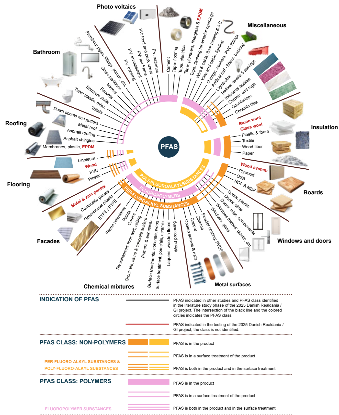
Figure 4. The PFAS circle shows construction products that may contain PFAS, based on a literature review of, among other things, tests and patent analyses from a number of published reports. Seven product types are marked in red, indicating, according to the project's test results, a potential PFAS content. The red lines do not indicate PFAS classes, in contrast to the black lines for the other product types. F-gases are not included in the PFAS Circle. The PFAS Circle was developed and quality-assured by Henning Larsen Architects and Søren Jensen Consulting Engineers A/S. Copyright PFAS CIRCLE 2025. Images used in accordance with Rambøll Adobe Stock Licence. Graphics by Anna-Mette Monnelly and Martha Lewis.
