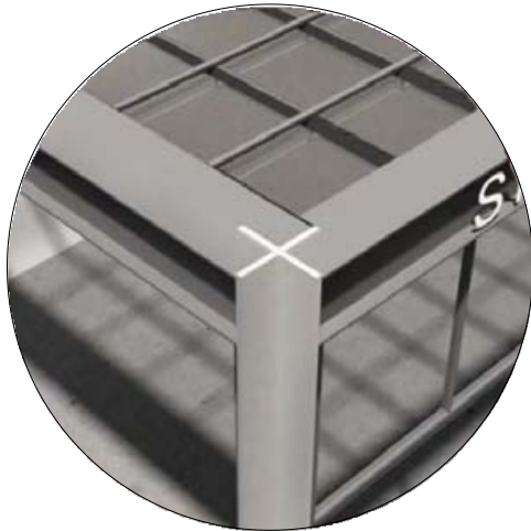
COLUMN TO SIGNAGE BEAMS & GLASS CEILING
