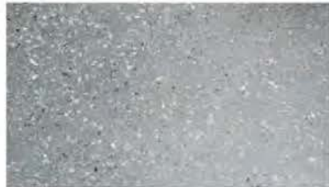
Upcycled concrete with aggregates of reused concrete.
