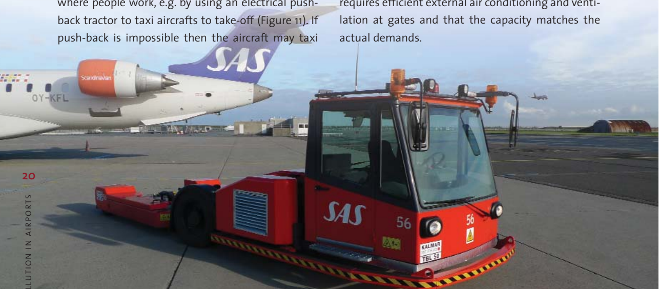
Figure 11: Electrical push-back tractors eliminate local emissions
